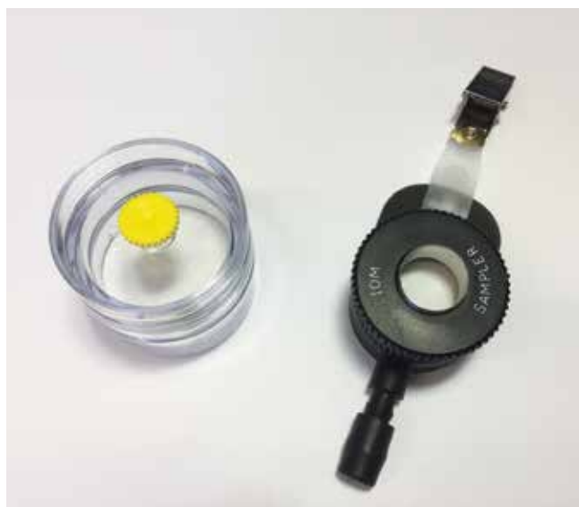
Figure 1. 37mm Air Sampling Cassette and IOM Inhalable Dust Sampler.
