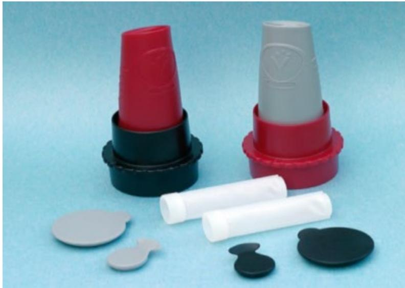
1. Insert the nylon filter into the DUSTREAM<sup>®</sup> collector and attach the collector to the vacuum cleaner tube.
